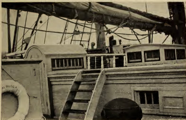
Cabin trunk and after details, barque "CALBURGA." (Photo by the author.)
