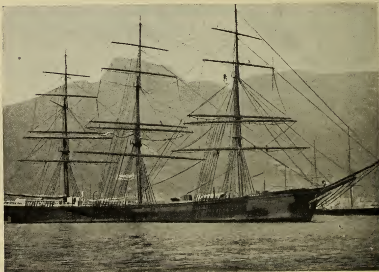
Ship "CANADA," in Table Bay, South Africa. The original built masts have been replaced by iron lower masts, and skysail yards have been discarded.
